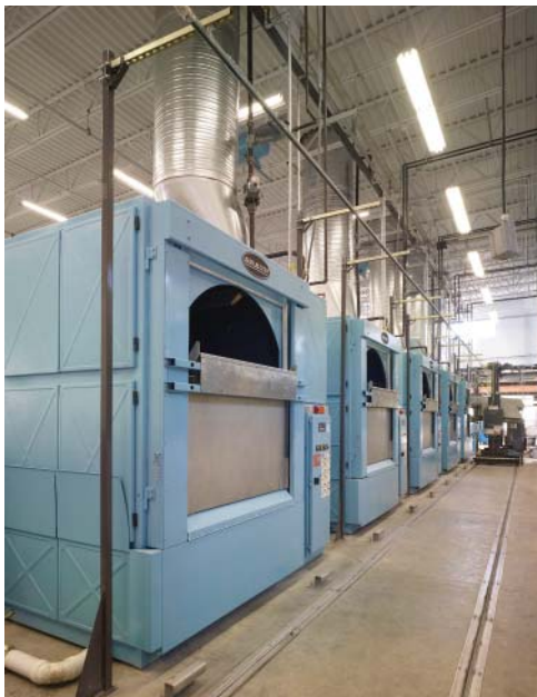
A shuttle system (at center/right) services these five 500 lb. dryers with two-batch, two-cake storage and transport, thus saving labor and improving throughput efficiency.
