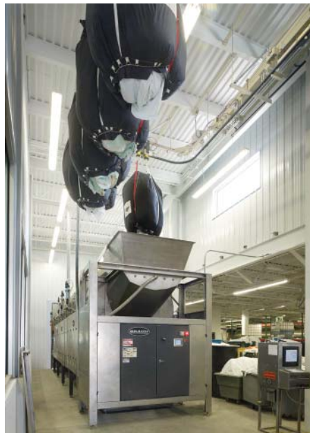
This tunnel with 14, 220 lb. compartments can process 6,600 lbs. per hour and has internal water- and energy-recovery systems that optimize resource conservation.
